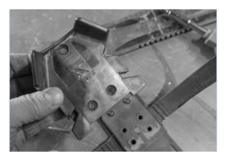
Put the top plate on and push it into place. Make sure the toe strap is still located properly, and put the screws in, this will keep all the parts in place.
