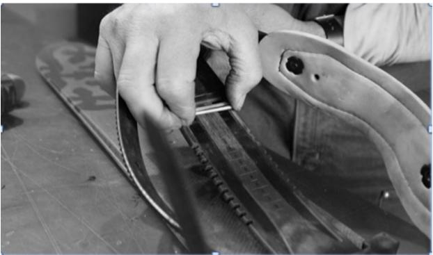
Finally, pinching in the steel adjustment tangs on the heel plate, slide the plate back off the old flex strap and then onto the new one.
