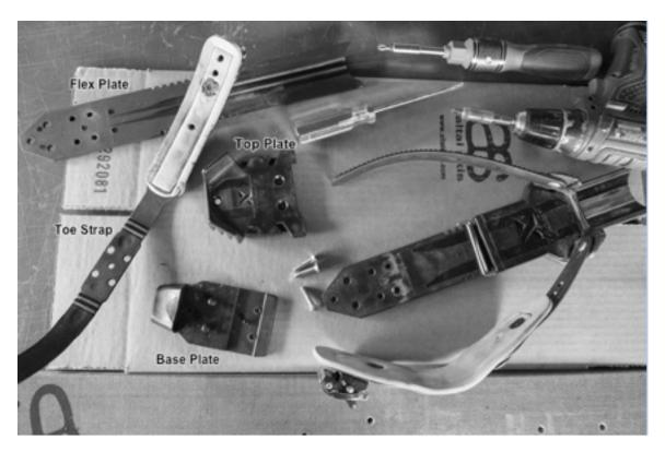
First, unscrew the 3 screws that hold the binding onto the ski. Remove them from the binding as well. The top plate (that your foot sits on) will come off easily.
